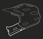
Press chinbar buttons with your thumbs to release and rotate chinbar upwards.
