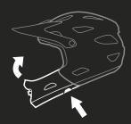
Pull chinbar up and away to disengage it from the helmet.
